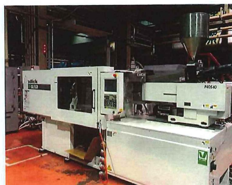
Fig. 4 Injection molding machine image
