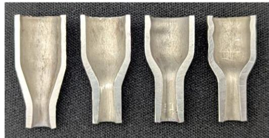
(a) 条件A ( $\phi = 15^\circ$ ) (b) 条件D ( $\phi = 20^\circ$ ) (c) 条件B ( $\phi = 25^\circ$ ) (d) 条件C ( $\phi = 30^\circ$ )
